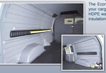
The EconoCargo® system protects your investments in your work van and your cargo, preventing dents and scratches over years of use. Molded-to-fit HDPE wall panels with protective ribs last the life of the vehicle, and thermal insulation improves climate control and reduces road noise.
